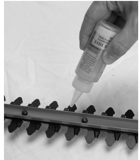
Figure 4-3: Oiling cutter blades
